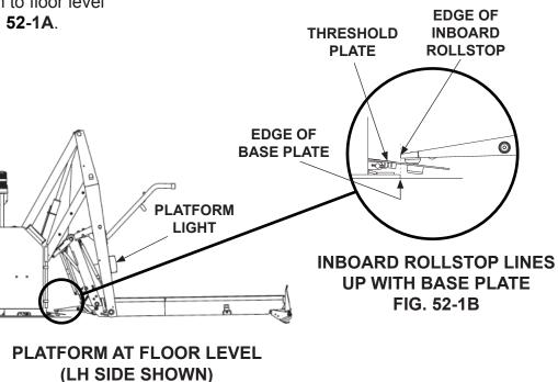
2. Inspect the threshold plate. The edge of the inboard rollstop should line up with the edge of the base plate as shown in FIG. 52-1B.
